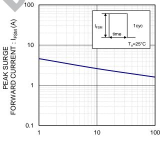
$$\label{eq:time_to_time} \begin{split} & \text{TIME: t (ms)} \\ & \text{I}_{\text{FSM}}\text{-t CHARACTERISTICS} \end{split}$$
